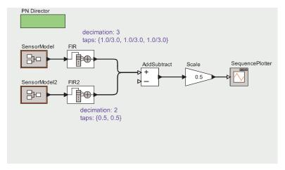
The non-default parameters of the FIR filters are shown in the figure. In this model, instead of discarding sensor data, each output of the downsampling filter is the average of either 3 or 2 neighboring samples. The result of running this model is shown below:
