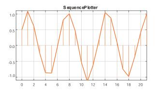
This technique will work for any sample rates, as long as they are known *a priori*. However, this only goes as far as generating a reasonable plot. The samples are not actually combined in any useful way. In particular, even samples with the same time stamp are not combined, and instead appear in the plot as samples at the same time, but with different values.  $\Box$
