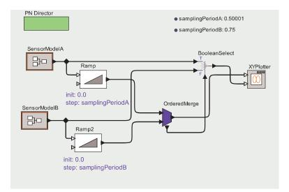
In this solution, the two Ramp actors are used to generate a sequence of time stamps corresponding to the times of the original samples. The OrderedMerge will order these samples. Its output down the bottom tells us which input received each output that is produced. That signal can be used to merge the two sensor streams using a Select actor. The result of running this model is shown below:
