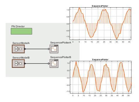
The plots show the (slightly noisy) sinusoids plotted vs. the sample number. Their frequencies (in cycles per sample) are, in fact, different, despite the fact that the SensorModel components purport to produce sinusoids with the same frequency. In cycles per second, the frequencies are roughly the same, although since PN has no time in its semantics, we have no assurance that the samples are generated at the rate we have indicated.  $\Box$
