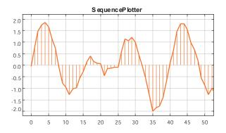
Notice that the plotted signal is not representative of the signal that the sensor models are sensing, which is a simple sinusoid. Instead, it is the sum of two sinusoids with different frequencies (plus noise). The AddSubtract actor is forcing the samples synchronize, adding one from each signal to get the result.
