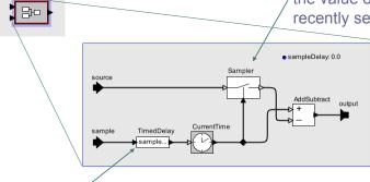
The TimedDelay actor transfers every input event to the output with a fixed increment in the time stamp. Here, the value is sampleDelay, a parameter of the composite actor.
