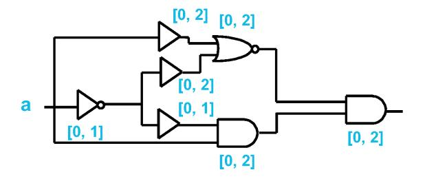
Delay of 6 for the above circuit for transition model (longest path that can propagate a transition)
