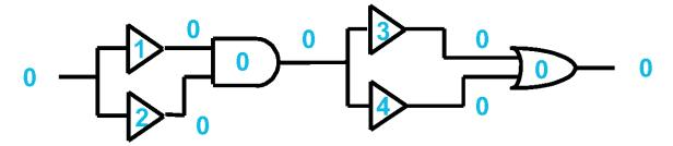
Path of length 6 is statically co-sensitized Delay of circuit is 5 (as observed earlier)
