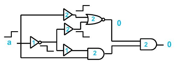
Transition delay is 0, for both input transitions. Consider the "faster" circuit
