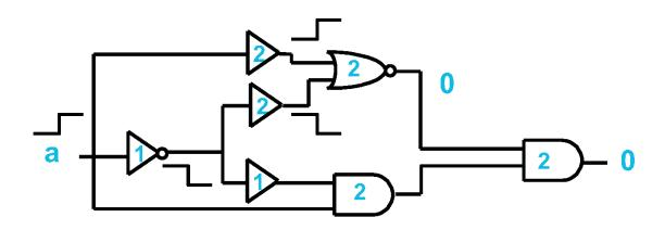
Transition delay is 0, for both input transitions. Consider the "faster" circuit
