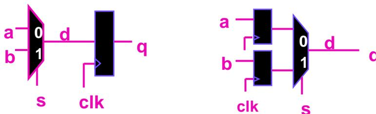
Circuits are equivalent but it is not possible to show that they are equivalent using Boolean equivalence
